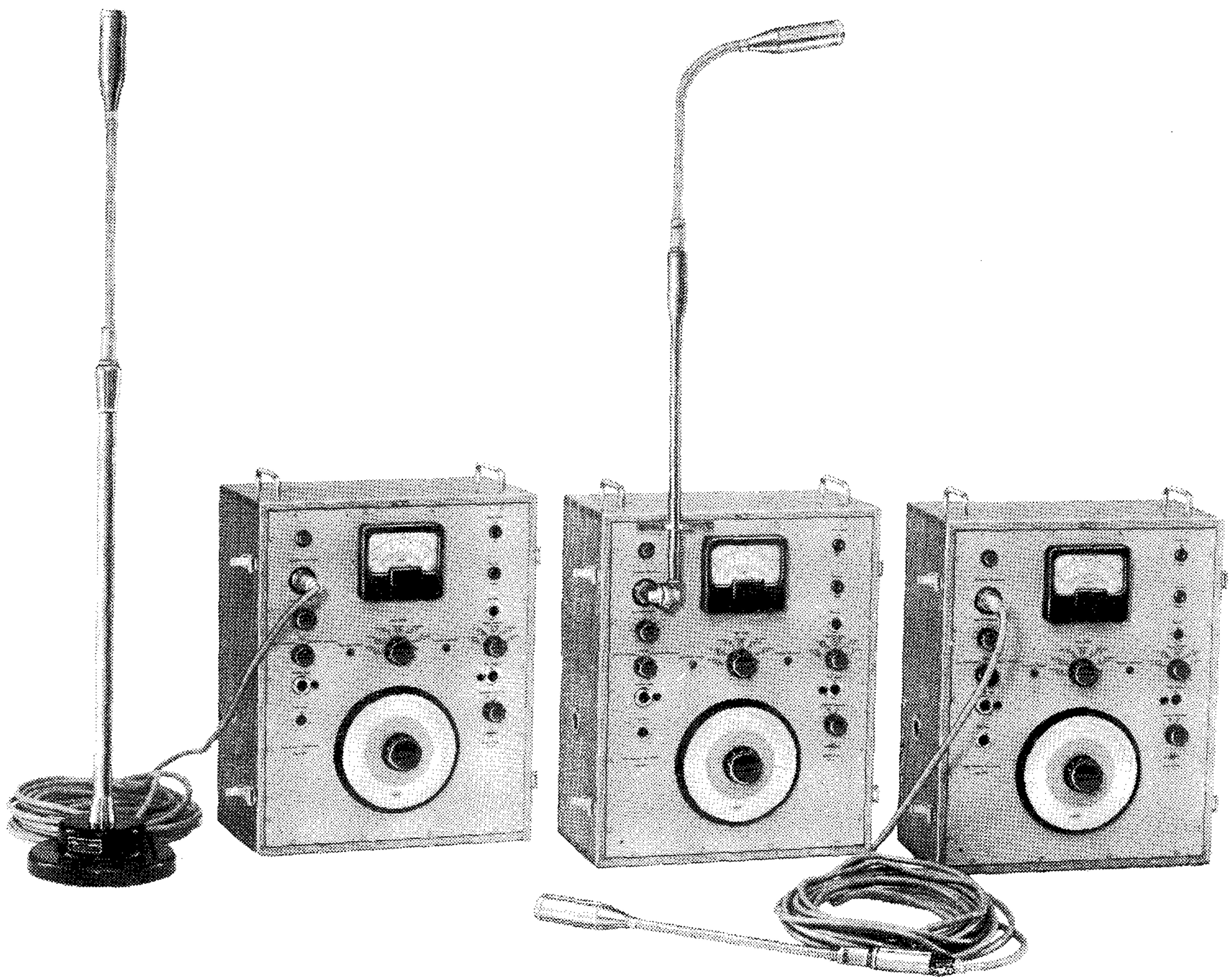
Fig. 17. Photo of the Condenser Microphone Type 4111 connected to the Spectrometer. Left: Floor Stand Type 4112, Middle: Extension Rod Type 4115, Right: Extension Cable 4114.
